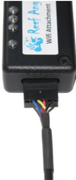
3. Connect the 8 pin connector to the Serial TTL port of the Reef Angel Head Unit.
